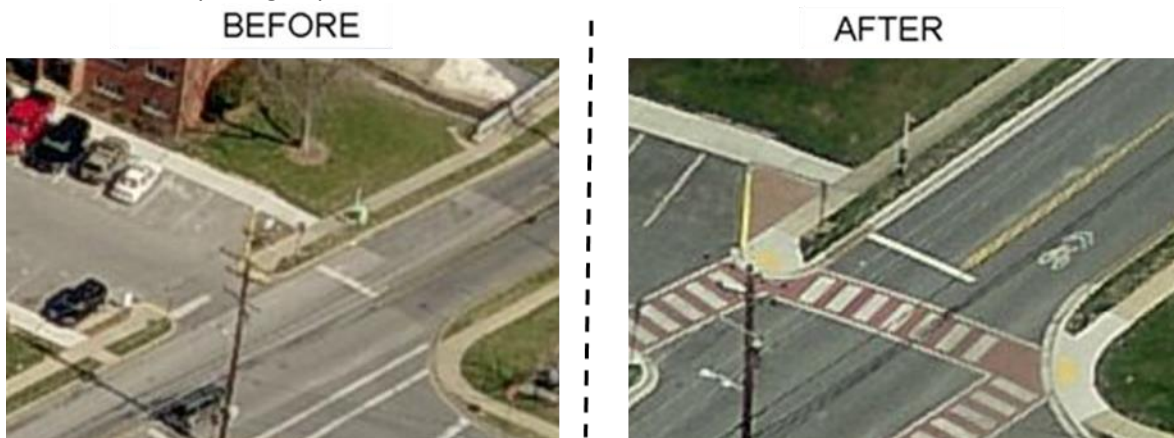
Figure 14: Before and After Signage/Striping Improvements for 4th St.
