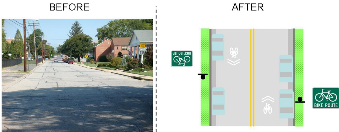
Figure 18: Before and After Signage/Striping Improvements for 8th St.
