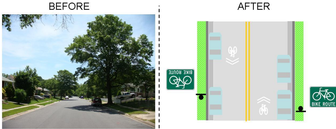
Figure 45: Before and After Signage/Striping Improvements for White Way.
