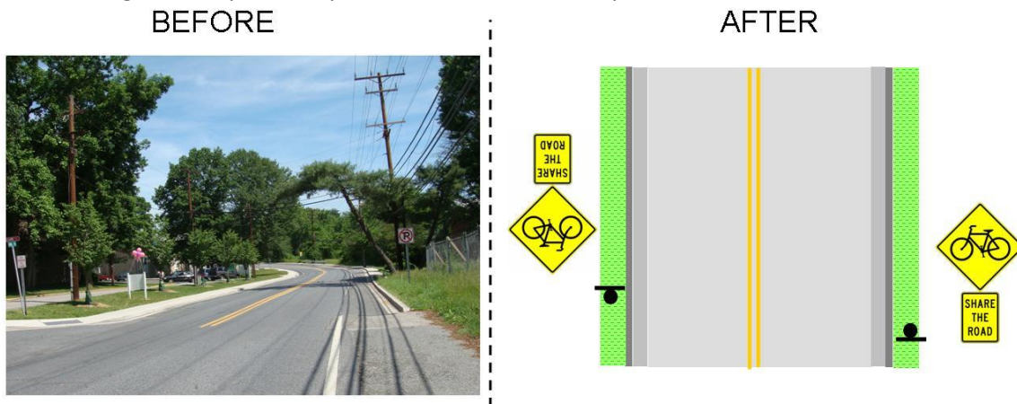
Figure 22: Before and After Signage/Striping Improvements for Bowie Rd.
