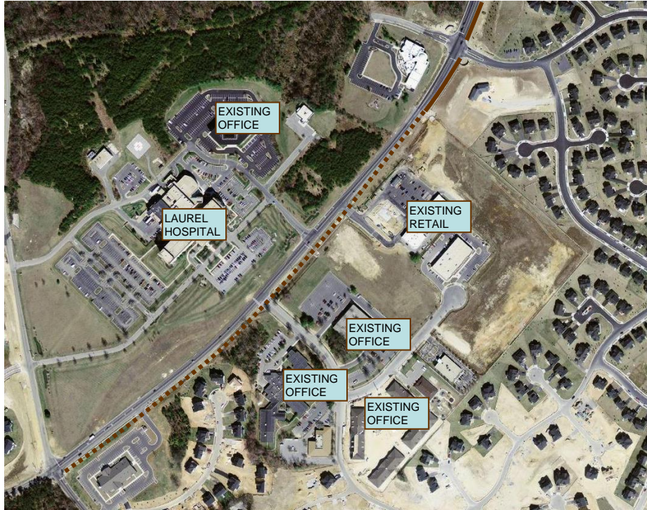
Figure 43: Extension of Pedestrian side trail – shown as a dotted brown line - along Van Dusen from Killbarron Road in the north to Contee Road in the South.
