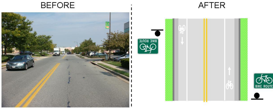
Figure 33: Before and After Signage/Striping Improvements for Laurel Place
