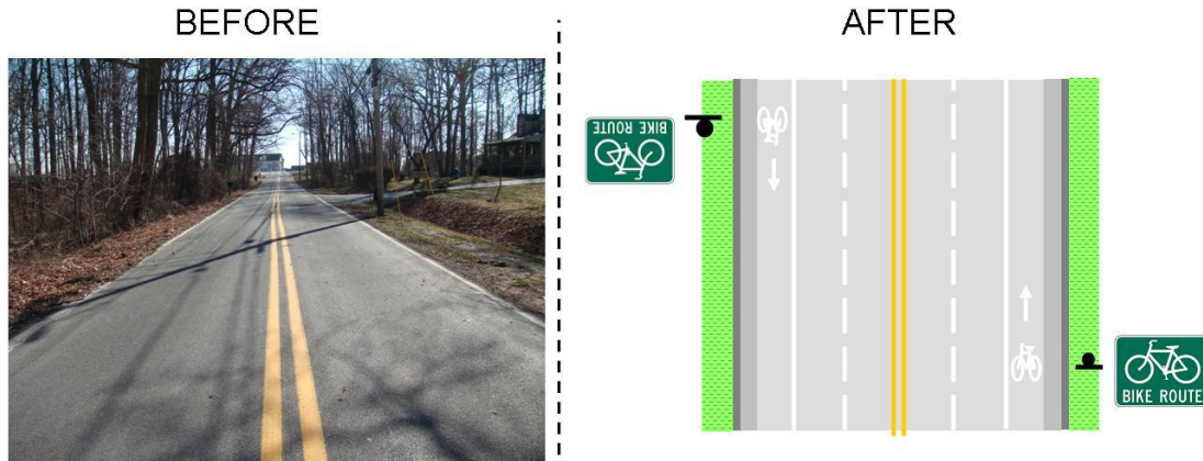
Figure 23: Before and After Signage/Striping Improvements for Cherry Lane.
