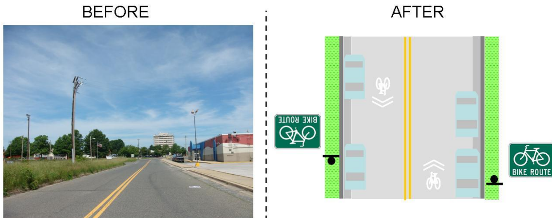
Figure 36: Before and After Signage/Striping Improvements for Marshall Ave.
