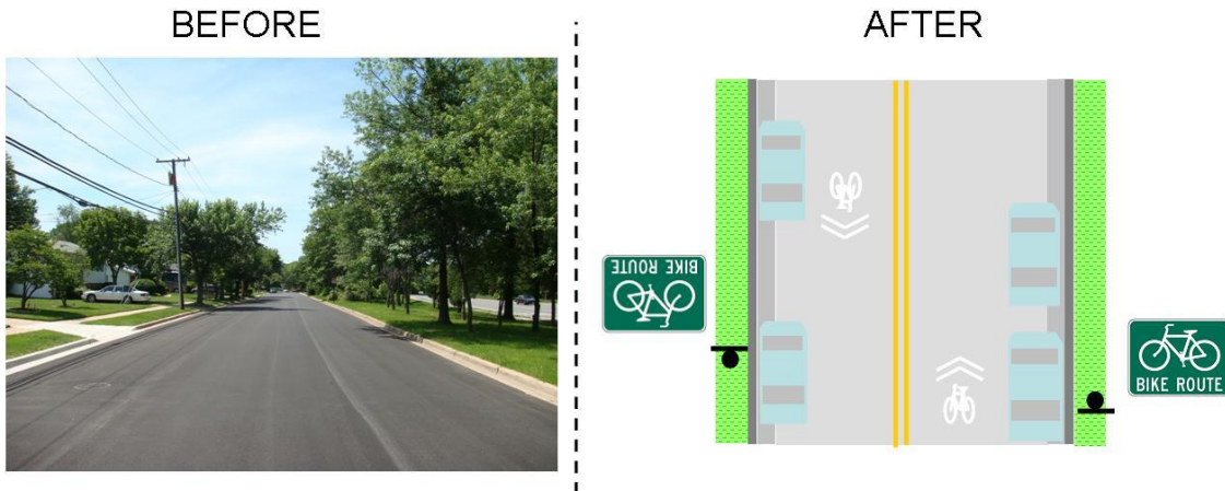
Figure 34: Before and After Signage/Striping Improvements for Laurelton Dr.
